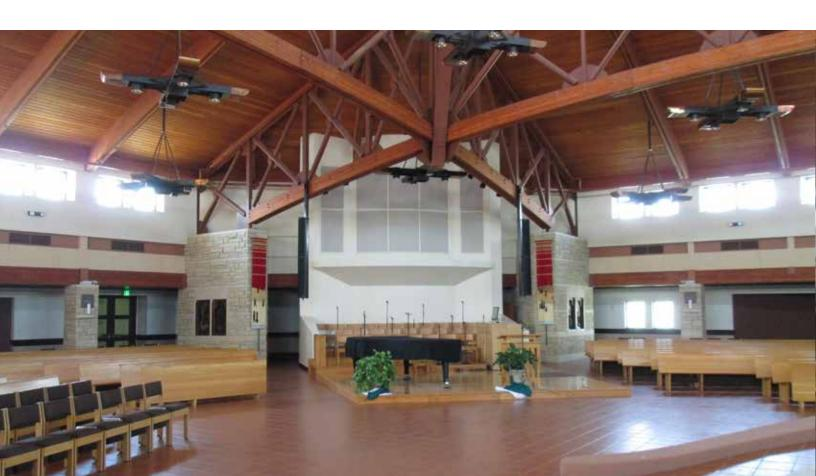
As Yost explains, the room's circular design and abundance of hard, reflective surfaces presented a number of challenges, and the existing distributed PA's speakers were aimed almost straight down at the tile floor, creating uncontrolled reflections that exacerbated the room's ringing 3.5-second reverberation time.
